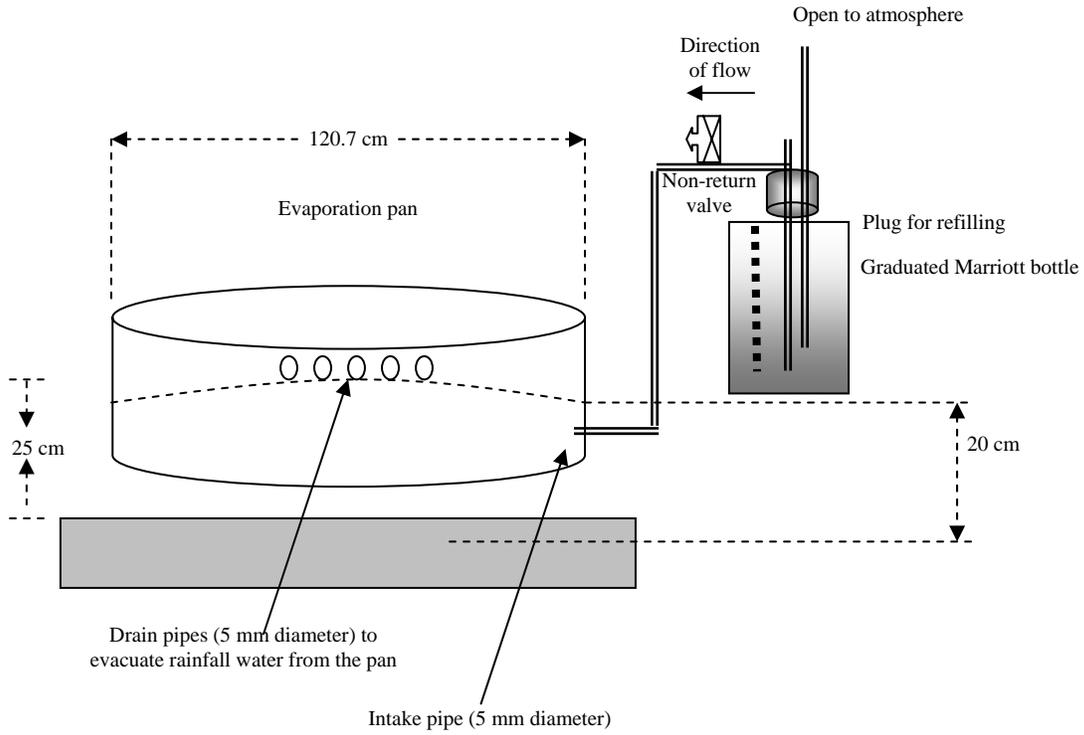
Figure 1: Schematic Diagram of the Modified Class- A Evaporation Pan
