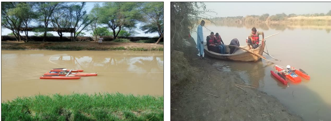
Figure 31: Discharge measurement through ADCP in canals
