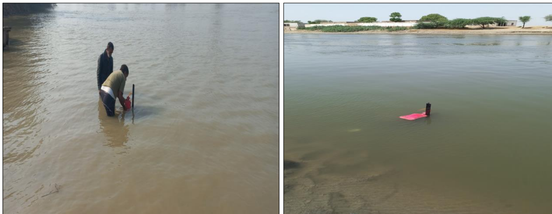
Figure 32: Seepage measurement in the active canal bed
