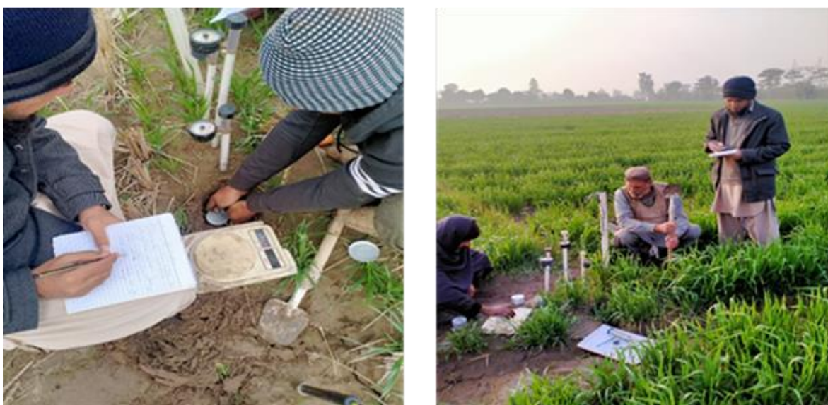
Figure 7: Soil sampling and recording tensiometer reading for soil moisture determination
