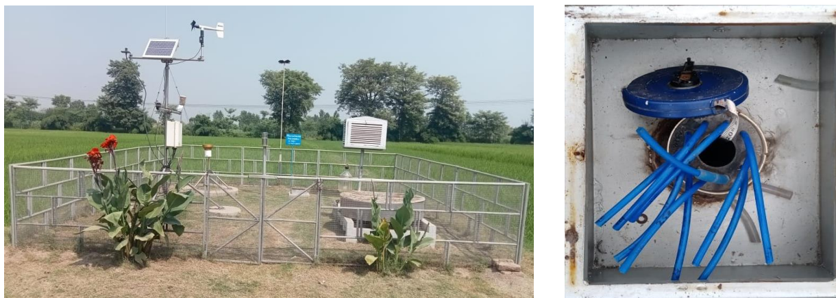
Figure 2: Climatic data observatory setup and piezometer/multi level observation well
