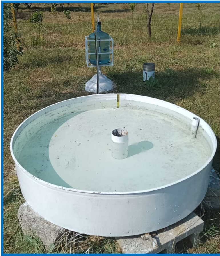
Figure 10: A view of the evaporation pan with Mariote Bottle
