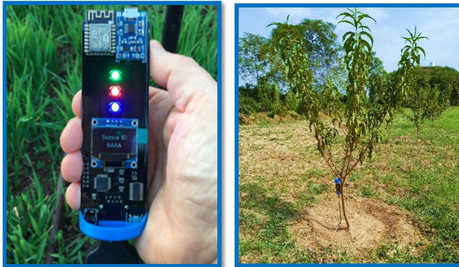
Figure 12: A view of the Chameleon field reader and sensor installed in field
