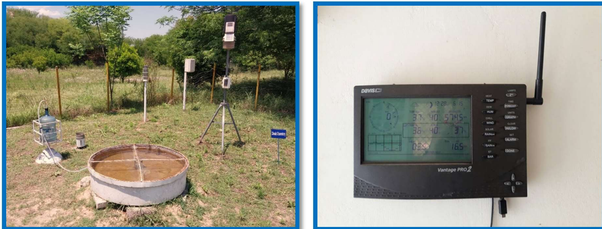
Figure 8: Weather station installed at the farm and receiver
