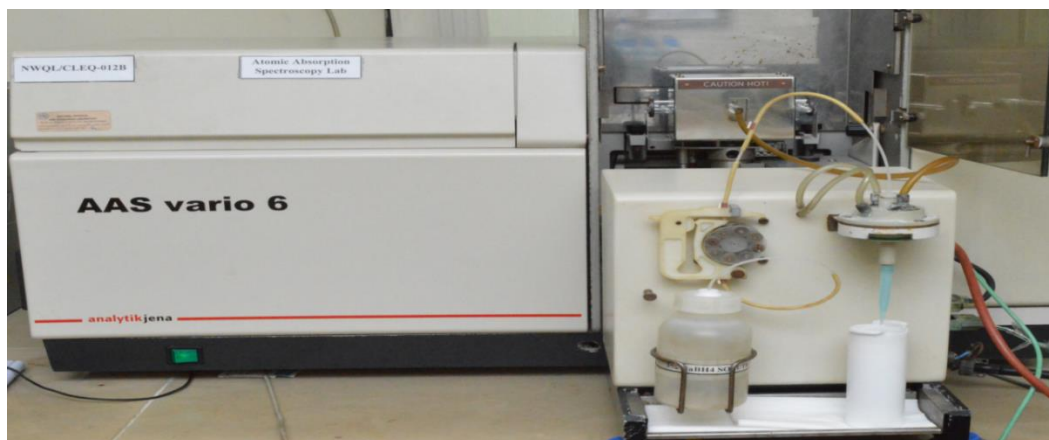
Figure 9: Electrical Heated Optical Cell with Batch Flow System in HGAAS
