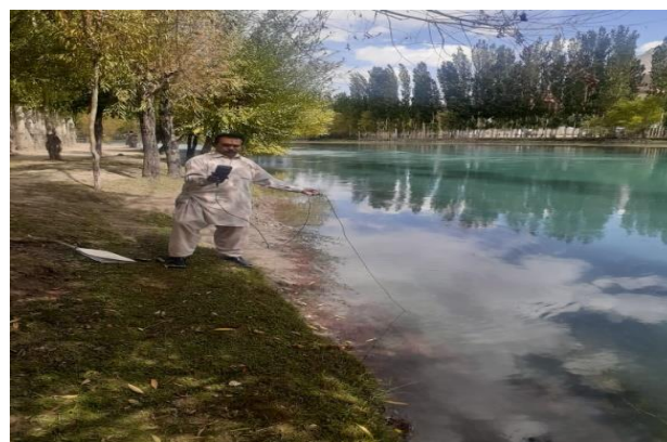
Figure 12: Determination of onsite DO and record keeping
