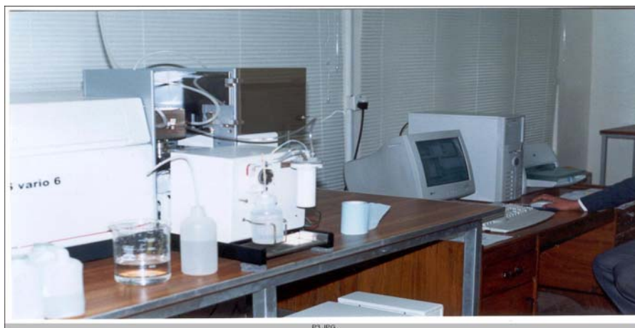
Fig.-1: Mercury Hydride System of Atomic Absorption Spectrophotometer (AAS)
