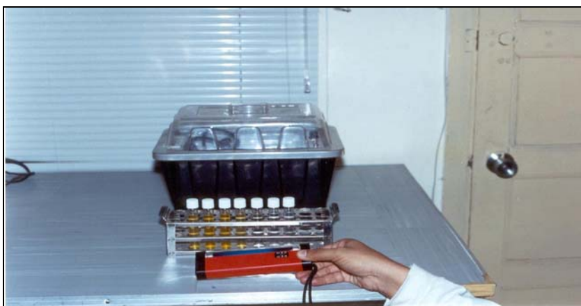
Determination of E-Col Count by MPN Method
